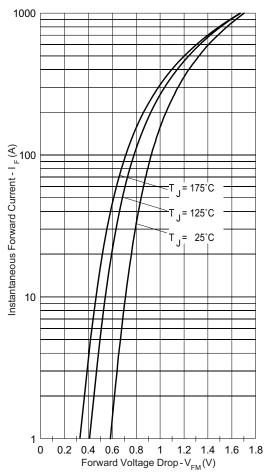
Fig. 1 - Maximum Forward Voltage Drop Characteristics
