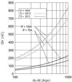
Fig. 8 - Typical Stored Charge vs. dl<sub>F</sub>/dt
