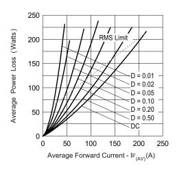
Fig. 6 - Forward Power Loss Characteristics
