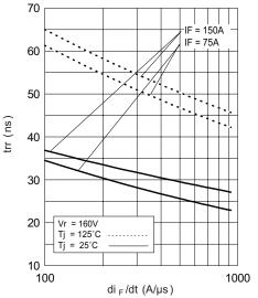
Fig. 7 - Typical Reverse Recovery Time vs. dl<sub>F</sub>/dt
