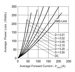
Fig. 6 - Forward Power Loss Characteristics
