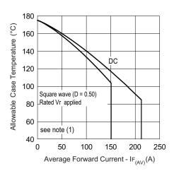
Fig. 5 - Maximum Allowable Case Temperature vs.
