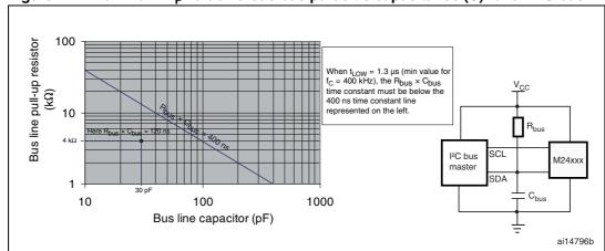
Figure 4. Maximum R<sub>p</sub> value versus bus parasitic capacitance (C) for an I<sup>2</sup>C bus
