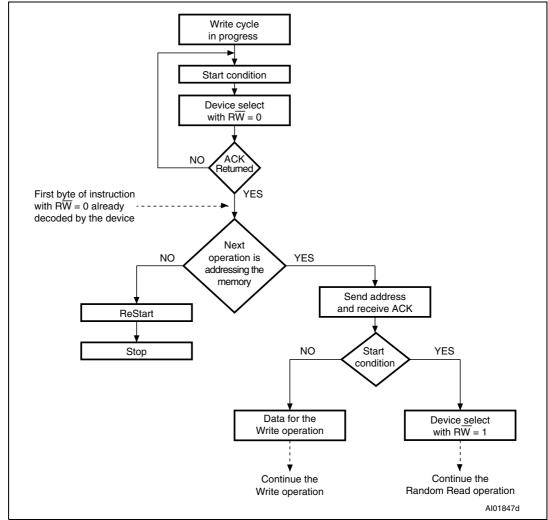
Figure 9. Write cycle polling flowchart using ACK
