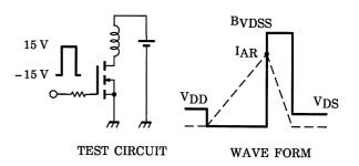
$$\begin{aligned} &R_G = 25~\Omega \\ &V_{DD} = 90~V,~L = 7.35~mH \end{aligned} \quad E_{AS} = \frac{1}{2} \cdot L \cdot I^2 \cdot \left( \frac{BVDSS}{BVDSS - VDD} \right)$$
