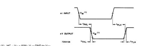
(1) HC :  $V_M$  = 50%;  $V_I$  = GND to  $V_{CC}$ . HCT:  $V_M$  = 1.3 V;  $V_I$  = GND to 3 V.
