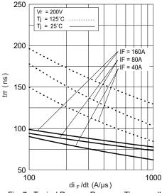
Fig. 7 - Typical Reverse Recovery Time vs.  $dI_F/dt$
