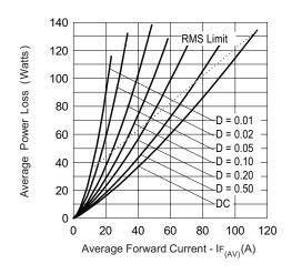
Fig. 6 - Forward Power Loss Characteristics
