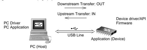
The USB is used to transmit information that has the following configuration:
