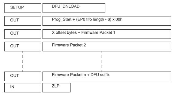
The Host sends a DFU\_DNLOAD request with the wLength field cleared to 0 to the device to indicate that it has completed transferring the firmware image file. This is the final payload packet of a download operation.
