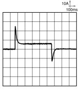
6-(2). Electrical life test (Motor lock) Sample: ACT212, 3pcs. Load: 25A 14V DC
