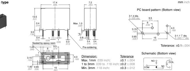
\* Dimensions (thickness and width) of terminal specified in this catalog is measured before pre-soldering. Intervals between terminals is measured at A surface level.
