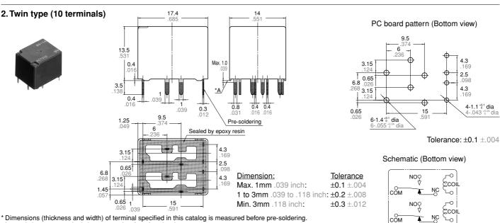
Intervals between terminals is measured at A surface level
