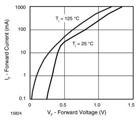
Figure 3. Forward Current vs. Forward Voltage
