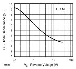
Figure 4. Diode Capacitance vs. Reverse Voltage
