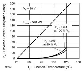
Figure 1. Max. Reverse Power Dissipation vs.
