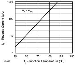
Figure 2. Reverse Current vs. Junction Temperature
