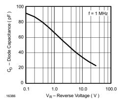
Figure 6. Diode Capacitance vs. Reverse Voltage
