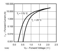
Figure 2. Forward Current vs. Forward Voltage
