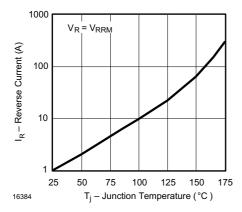
Figure 4. Reverse Current vs. Junction Temperature
