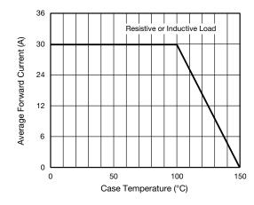
Fig. 1 - Forward Current Derating Curve
