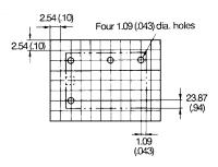
Single winding types, 2-pole G6CU-2117P-US, G6CU-2114P-US
