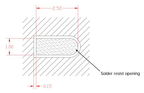
It is not recommended to place via or micro-via not covered by solder resist in an area of 0.3 mm around the pads unless it carries the same signal of the pad itself (see following figure).
