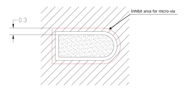
Holes in pad are allowed only for blind holes and not for through holes.
