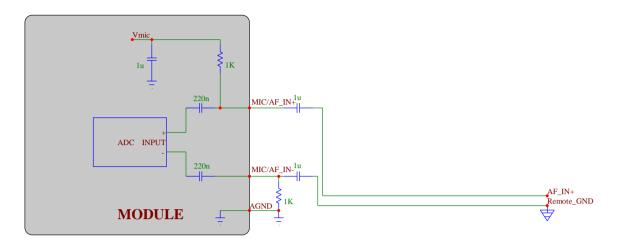
If the audio source is not a mike but a different device, the following connections can be done. Place a  $1K\Omega$  resistor to ground on the negative input, in order to get balanced the input; than connect the source via 1uF capacitor, so the DC current is blocked.
