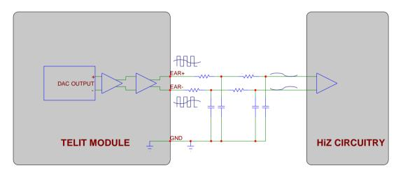
R-C filtering for HIGH impedance load.
