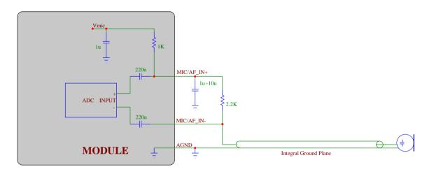
If a "balanced way" is anyway desired, much more care has to be taken to Vmic noise and ground noise; also the  $33pF-100\Omega$ -33pF RF-filter has to be doubled (one each wire).
