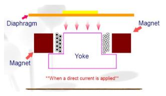
Drawing of the Magnetic Buzzer.
