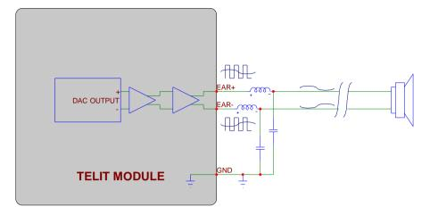
L-C filtering for LOW impedance load.
