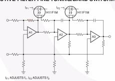
The linearity of resistance and the low offset voltage of the H11FXM allows the remote tuning or band-switching of active filters without switching glitches or distortion. This schematic illustrates the concept, with current to the H11F1M IRED's controlling the filter's transfer characteristic.
