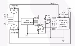
The optical isolation, linearity and low offset voltage of the H11FXM allows the remote multiplexing of low level analog signals from such transducers as thermocouplers, Hall effect devices, strain gauges, etc. to a single A/D converter.
