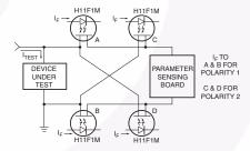
In many test equipment designs the auto polarity function uses reed relay contacts to switch the Kelvin Contact polarity. These reeds are normally one of the highest maintenance cost items due to sticking contacts and mechanical problems. The totally solid-State H11FXM eliminates these troubles while providing faster switching.
