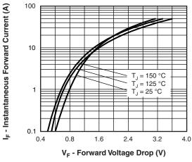
Fig. 1 - Typical Forward Voltage Drop Characteristics
