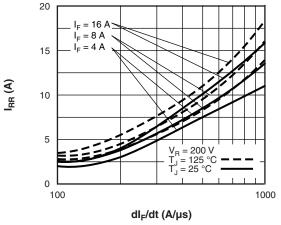
Fig. 6 - Typical Recovery Current vs. dl<sub>F</sub>/dt
