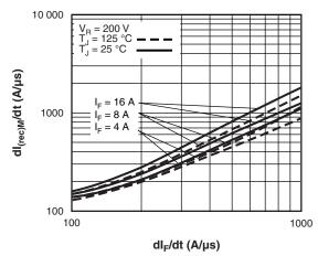
Fig. 8 - Typical dl<sub>(rec)M</sub>/dt vs. dl<sub>F</sub>/dt
