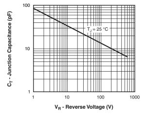
Fig. 3 - Typical Junction Capacitance vs. Reverse Voltage
