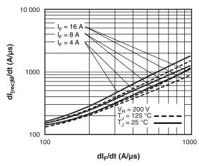
Fig. 8 - Typical  $dI_{(rec)M}/dt$  vs.  $dI_F/dt$
