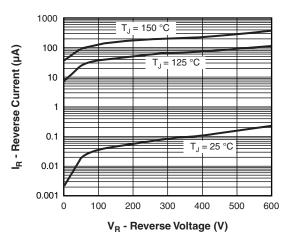
Fig. 2 - Typical Reverse Current vs. Reverse Voltage
