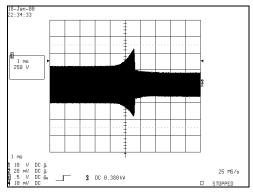
Waveform 2. Lamp voltage during preheat, ignition and run modes
