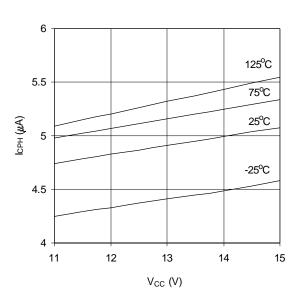
Graph 22.  $I_{CPH}$  vs  $V_{CC}$  vs Temperature (IR2156)  $V_{CPH} = 0V$
