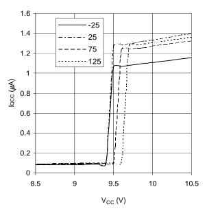
Graph 18.  $I_{QCC}$  vs  $V_{CC}$  vs Temperature (IR2156)  $V_{CCUV}$ -
