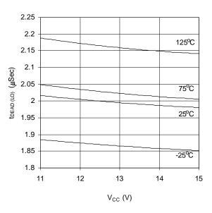
Graph 23.  $t_{DEAD}$  vs  $V_{CC}$  vs Temperature (IR2156) CT = 1nF
