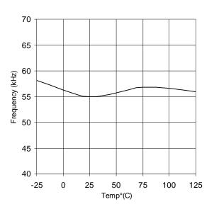
Graph 20.  $F_{OSC}$  vs Temperature (IR2156)  $V_{CPH} = 0V$
