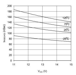
Graph 23. t<sub>RISE(HO)</sub> vs V<sub>CC</sub> vs Temperature (IR2156)
