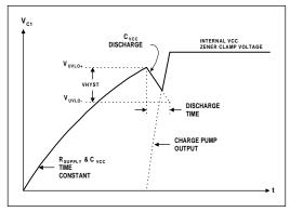
Figure 2, Supply capacitor (CVCC) voltage.
