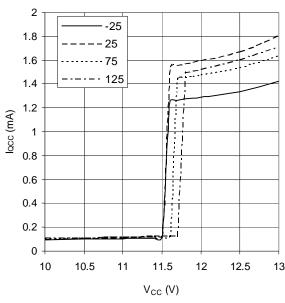
Graph 17.  $I_{QCC}$  vs  $V_{CC}$  vs Temperature (IR2156)  $V_{CCUV}$ +
