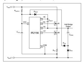
Figure 1, Start-up and supply circuitry.
