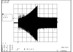
Waveform 1. Lamp filament voltage during preheat
