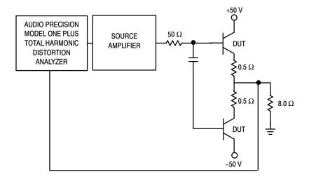
**Figure 17. Total Harmonic Distortion Test Circuit**
