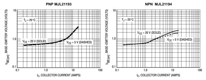
Figure 11. Typical Base-Emitter Voltage
