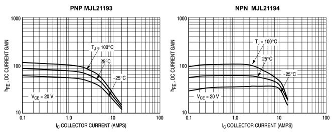
Figure 3. DC Current Gain,  $V_{CE} = 20 \text{ V}$
