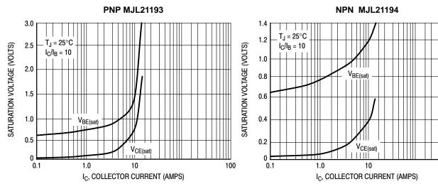
Figure 9. Typical Saturation Voltages
