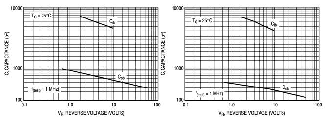
Figure 14. MJL21193 Typical Capacitance
