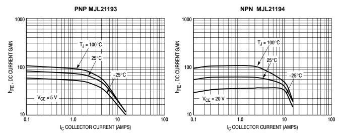
Figure 5. DC Current Gain, V<sub>CE</sub> = 5 V
