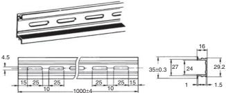
A total of twelve 25 × 4.5 elliptic holes is provided with six holes cut from each track end at a pitch of 10 mm.
