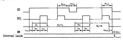
The data is latched at  $D_{\text{R}}\text{-H}$  and falling edge of the CE signal condition.
