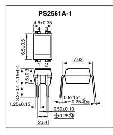
Lead Bending Type (Gull-Wing)
