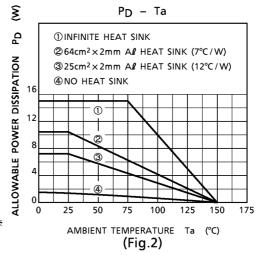
PD MAX =  $(16V-8V) \times (300\text{mA} + 100\text{mA} + 35\text{mA}) = 3.48\text{W}$  substituting PD max = 3.48W into expression (2), above,  $\theta$ HS is obtained as follows:
