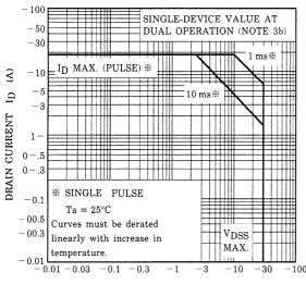
DRAIN-SOURCE VOLTAGE  $V_{DS}$  (V)
